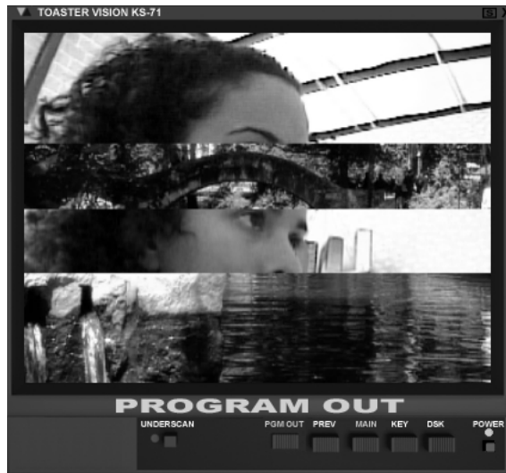
Figure 5.3. Display in Program Out mode with a Blinds DVE.
